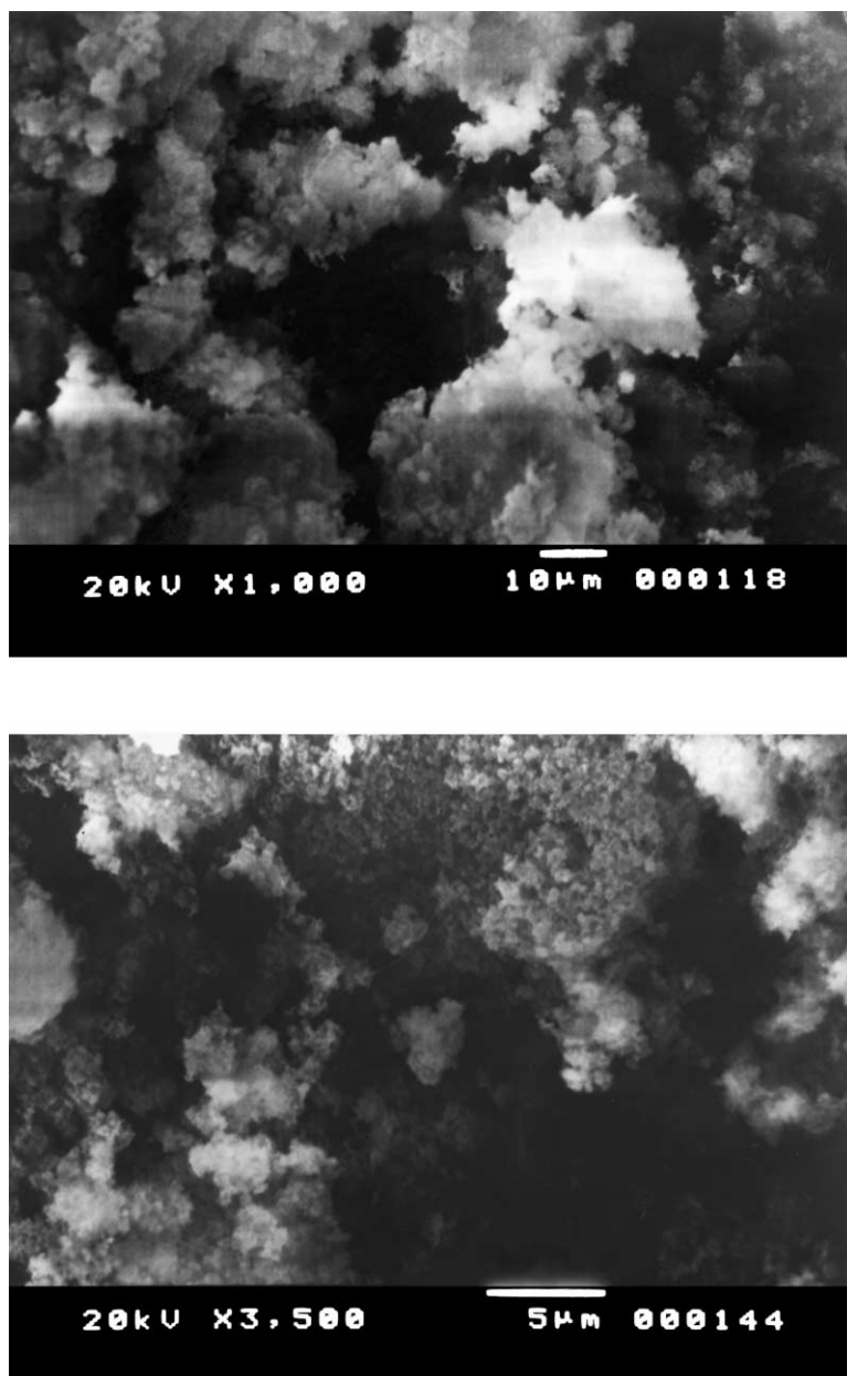
Fig. 6. SEM pictures of TH-MCM-41 (top) and U-MCM-41 (bottom).
