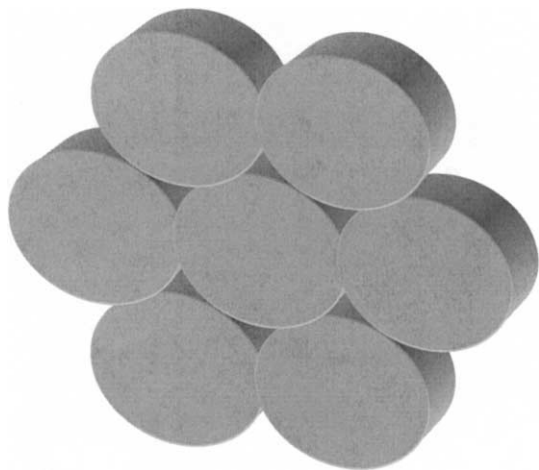
Fig. 1. MCM-41 after calcination showing the honeycomb structure of the silica matrix.
